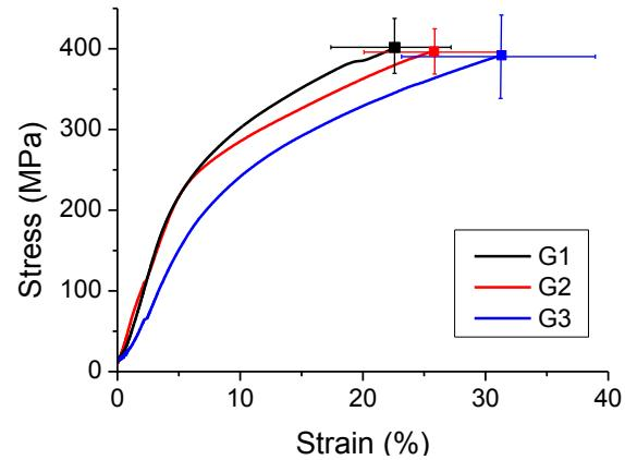
**Figure 3** Representative stress-strain curves of 3 grades of *B.mori* silks (from the middle layer of cocoons), error bars show the standard deviation of breaking strain and stress of 15 samples.
