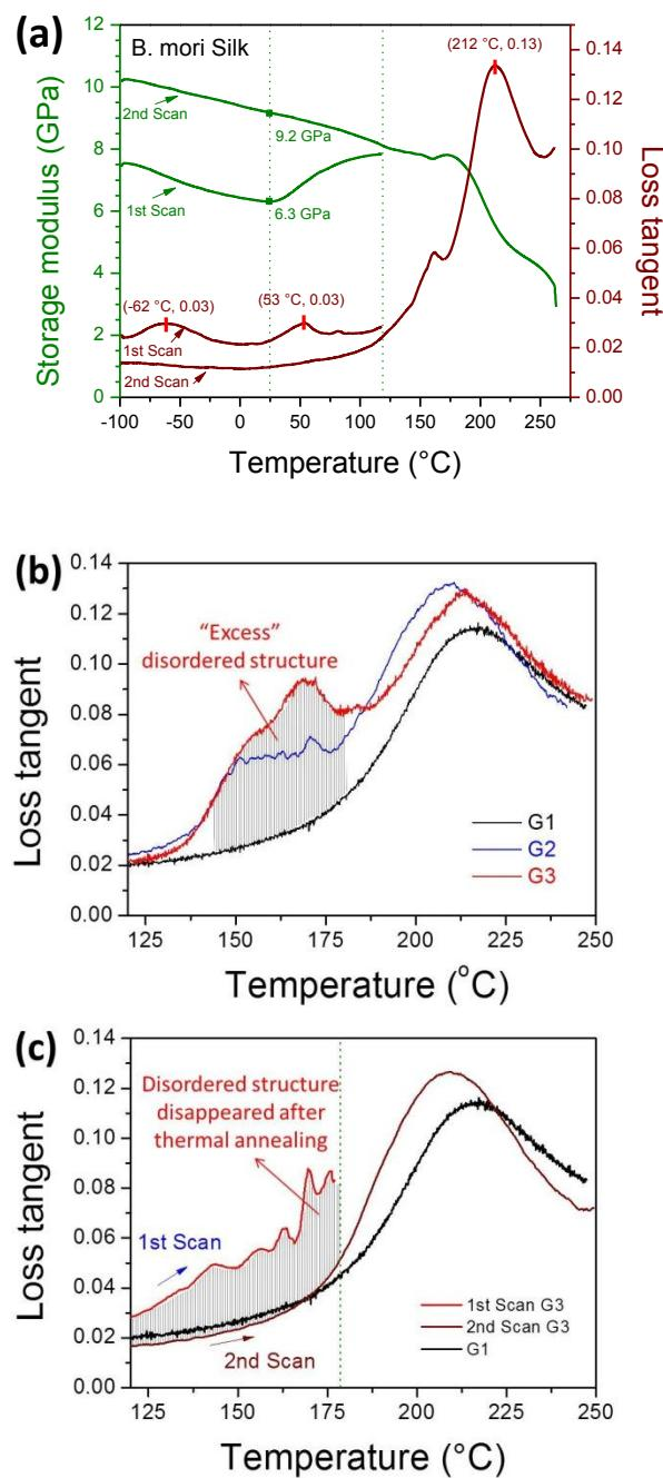
**Figure 4** (The figures are reproduced from [5]) Dynamic mechanical properties of silks from tests: DMTA cyclical temperature scan of G1 silk (a); DMTA temperature scans of the three grades G1, G2 and G3 (b); the annealing temperature scan to 180 °C of G3 (c).
