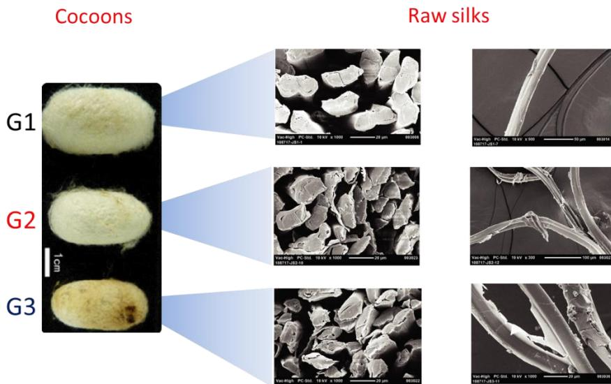
**Figure 2** Photographs of the three cocoon grades are on the left, SEM images of the cross-sections are in the middle column, and surface/longitudinal views of the raw silks taken from the middle layer of the cocoons are shown on the right.
